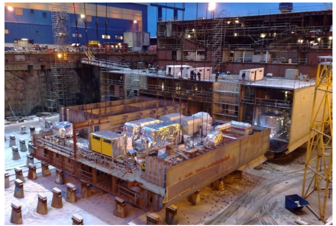
The CleanSea System installed on the ship's hull during ship building. The biological treatment basins are located in the far corner of the block.
